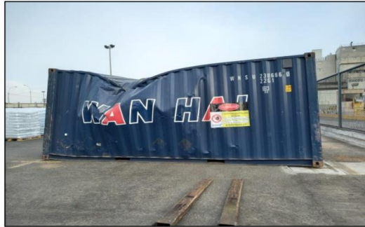
Panel of right side distorted (bulged out) due to heavy dent on the roof, affecting also the top side rail.
