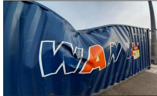
Panel of right side distorted (bulged out) due to heavy dent on the roof, affecting also the top side rail.
