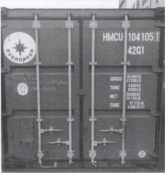
The photograph shows the side of a dark-colored container with the Evergreen logo (a compass rose) on the left. On the right, there is a white label with the following text: HMCU 1041051, 42G1, GROSS 20,480 KG / 67,200 LB, TARE 3,640 KG / 8,030 LB, NET 26,840 KG / 59,170 LB, CUBE 67.7 CU M / 2,390 CU FT. The container shows signs of wear and damage on its side panels.
