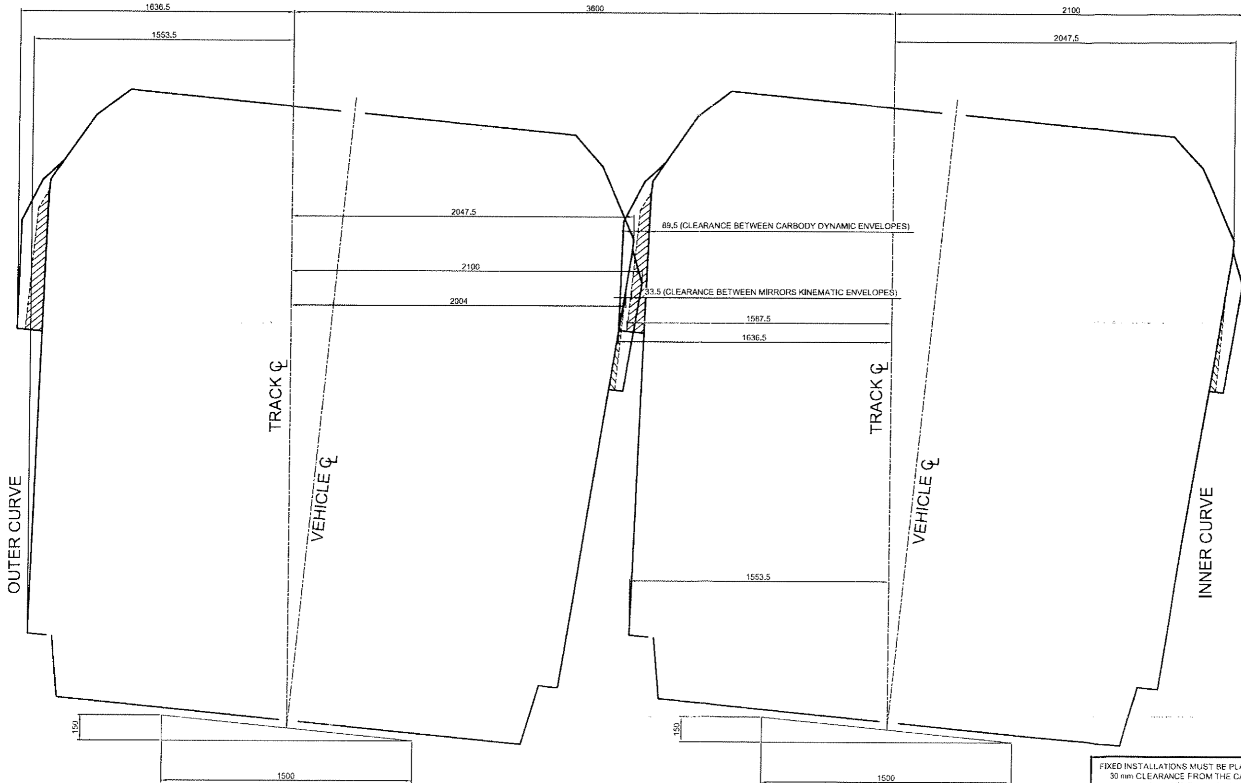
MINIMUM ACCEPTABLE DISTANCE BETWEEN TRACK CENTER LINES ON 250 m CURVE WITH CANT 150 mm
